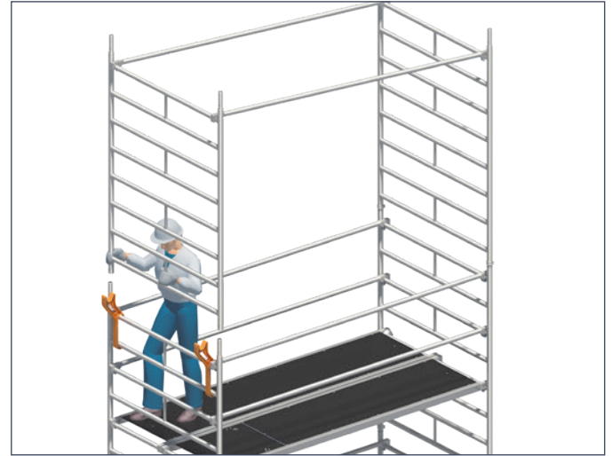
2. Swivel the ladder frame with guardrail upwards and fit it in place.
