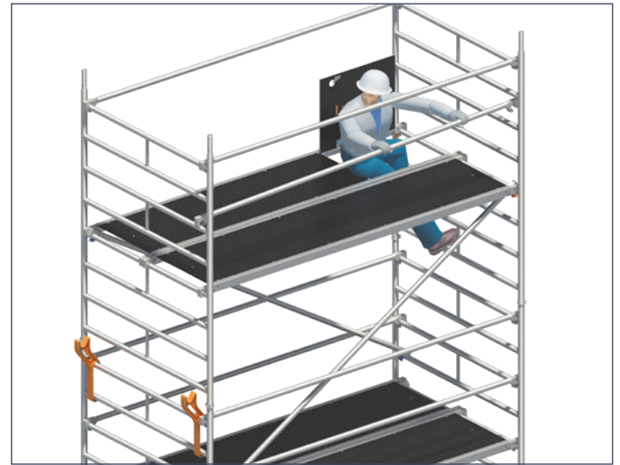
4. Assemble the intermediate rails from a secured position in the area of the access hatch.
